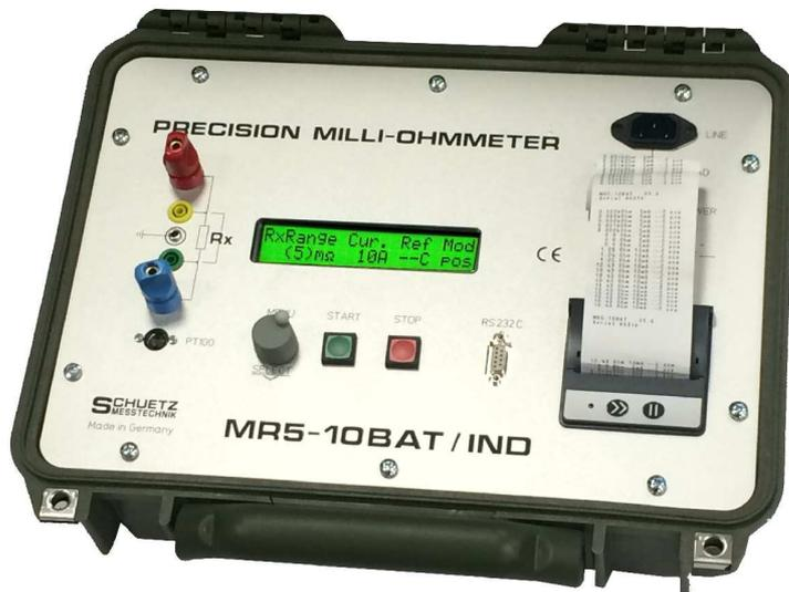
Accurate low resistance measurements can be handled with this battery driven MICRO-OHMMETER MR5-10BAT/IND. Measuring objects are fuses, bus bars, heating elements, circuit breakers, switch gears, relays as well as small inductive loads like motors, transformers, chokes etc.. The measuring object is connected due to the Kelvin/Thompson method with full 4 wire terminal connection. Current cable resistances are eliminated in this way.
